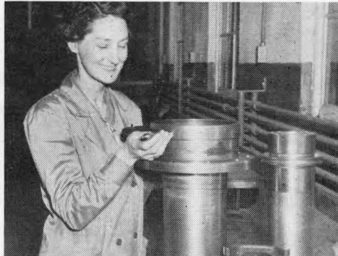
Woman war craftsman inspects with micrometer mounting for Oerlikon gun.
